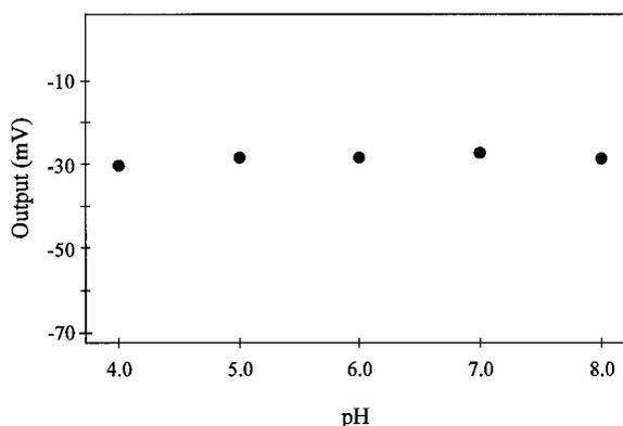
**Figure 4.** Effect of pH on  $\text{Cd}^{2+}$  microelectrode performance. The pH of five different 50  $\mu\text{M}$   $\text{Cd}(\text{NO}_3)_2$  solutions were adjusted over a range spanning from pH 4.0 to 8.0, using a series of buffers consisting of 10 mM Homopipes and 10 mM Tris added in the appropriate proportions to achieve the desired pH. The electrical output of the electrode was measured and then referenced to a 0 level, as described in Figure 1.
