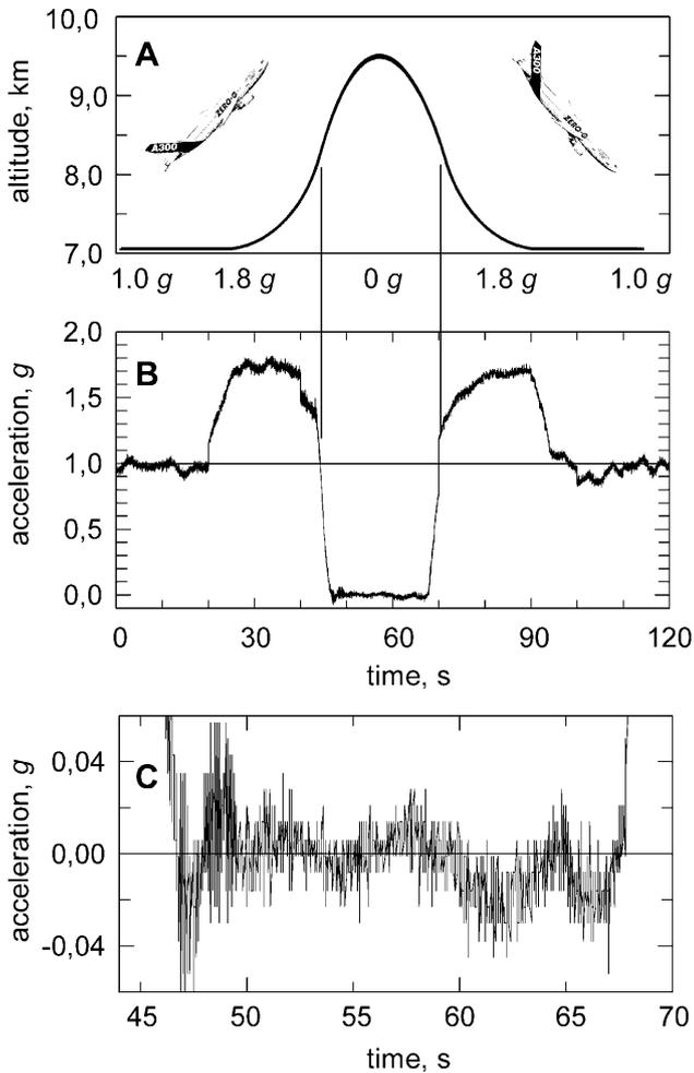
**Figure 3.** A, Trajectory of the airbus A300 ZERO G during a parabola flight. The vectors of the 1g and the 1.8g accelerations are always parallel to each other and to the plumb line, i.e. 90° relative to the floor of the airplane. B, Gravitational acceleration during flight parabolas expressed as multiples of  $g$  ( $9.82 \text{ m s}^{-2}$ ). C,  $g$ -values during microgravity (blow up of Fig. 3B).
