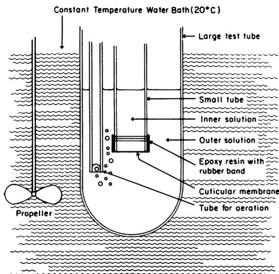
FIG. 1. Apparatus for measuring the permeability of a cuticular membrane to ions.
