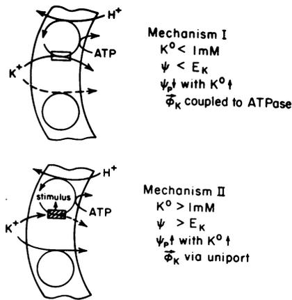
FIG. 6. Schematic model of electrogenic ATPase function and  $K^+$  influx at the plasmalemma of corn root cells under low and high  $K^{\circ}$  (mechanisms I and II of kinetic analysis). See text for description.
