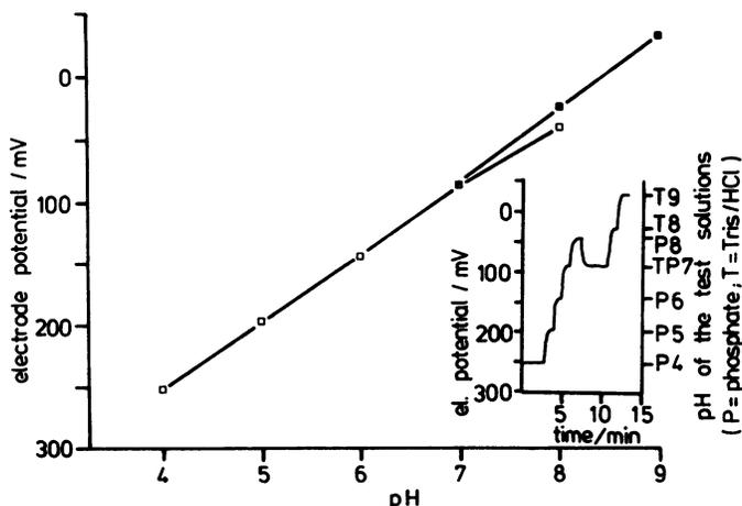
FIG. 1. Calibration curve of a typical ion exchanger pH microelectrode in sodium-phosphate buffer (□—□) and Tris/HCl buffer (■—■); other ions: 1 mM KCl, 1 mM CaCl<sub>2</sub>, 10 mM NaCl. Reference electrode: 3 M KCl. Inset: Original trace of electrode response to external pH.
