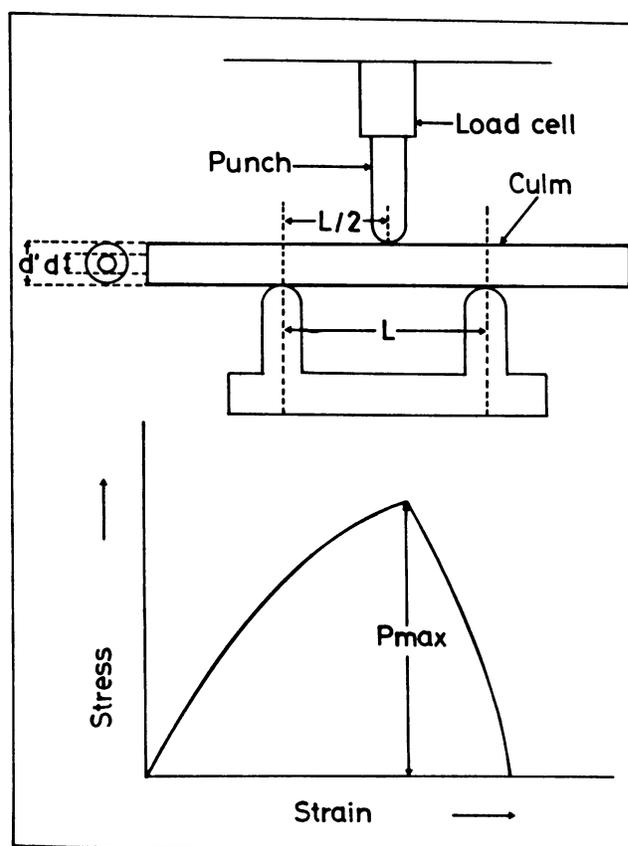
**Figure 1.** Measurement of maximum bending stress. Above, A 7-cm-long section of culm was placed on the edges 25 mm apart. The center of the culm was pressed by a 2-mm-diameter punch with a constant velocity of 50  $\text{mm min}^{-1}$ . Stress and strain were measured with an Auto-GRAPH, DCS-5000 (Shimadzu, Kyoto, Japan). Outer and inner diameter of the culm were measured microscopically. Below, A schematic form of a stress and strain curve.
