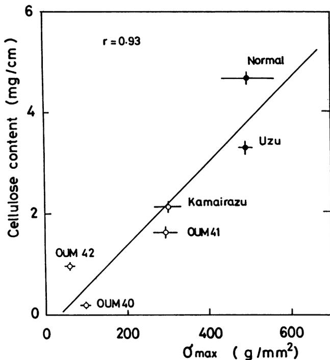
**Figure 4.** Correlation between cellulose content and maximum bending stress of fourth internodes of barley culms harvested in 1987. Maximum bending stress and cellulose content are shown in Table I and Table V, respectively.
