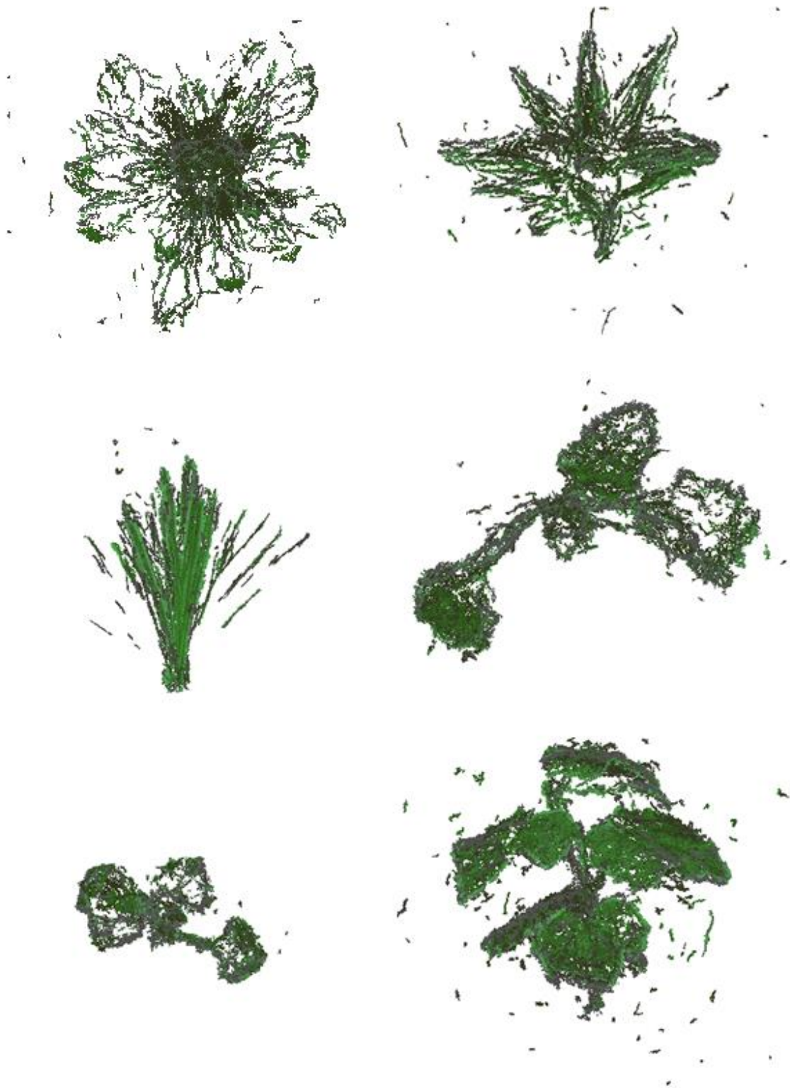
Supplementary Figure: Row one; experiment one and two, row two; experiment three and four, row three; experiment five and six. The supplementary figure illustrates the 3D reconstructions generated by the comparable imaging methods. The 3D points shown here highlight the lack of accuracy and detailed when compared to the AVC method proposed here.
